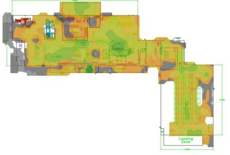
The detailed report would also help you to assess whether the data rates are adequate for the intended applications and the number of anticipated users. This survey is furthermore an invaluable tool in diagnosing problematic wireless networks by identifying hidden nodes, frequency interference, rogue APs and other wireless network hazards.
